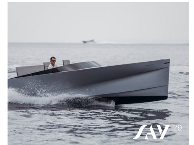
SAY Carbon Yachts designed a unique hydrodynamic "wave cutting" bow to ensure a comfortable and dry driving experience
